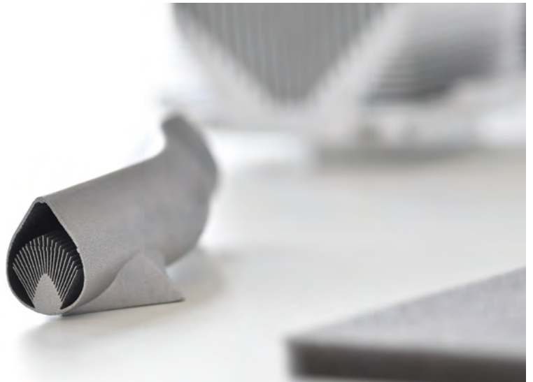
The ventilation element designed and printed by LIGHTWAY contains a lamella fan on the inside and could not be produced using conventional manufacturing methods. It replaces four aluminium parts approx. ten centimeters high (bottom picture). The additive robot ankle joint (right) is made of titanium.
