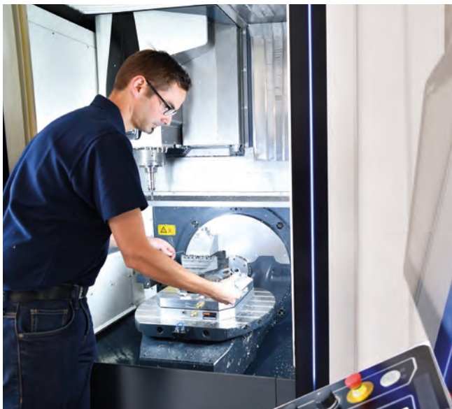
LIGHTWAY uses a five-axis metal-cutting machine to further process the titanium ankle joint for the robot at the Technical University of Munich.
